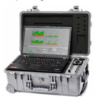
Liona is an online PD Spot Testing and PD location unit for cables and switchgear with advanced signal processing for detection of partial discharges in high noise environments.
