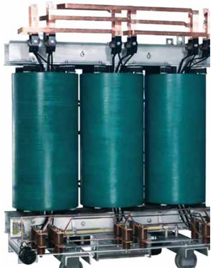
1600 kVA 10 KV / 3x1520 V DTR 101600 18 pulse rectifier transformer with phase shift+-20°
